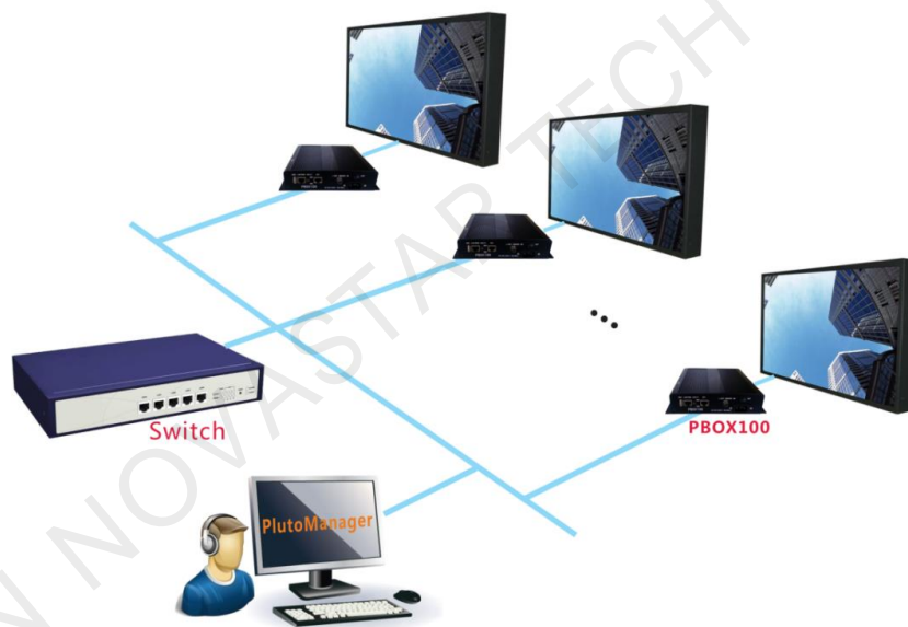
Fig. 5-9 All LED displays and control computers locate in the same LAN
