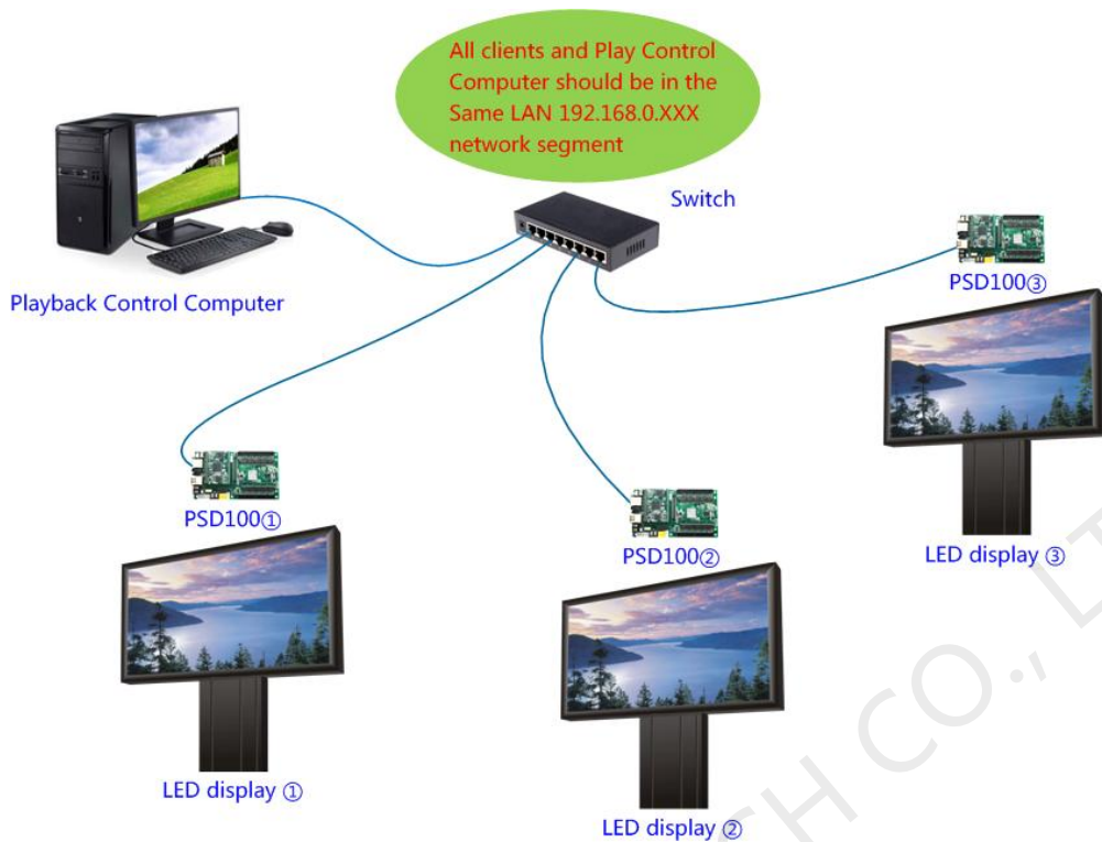
Fig. 2-1 All LED displays and control computers locate in the same LAN
